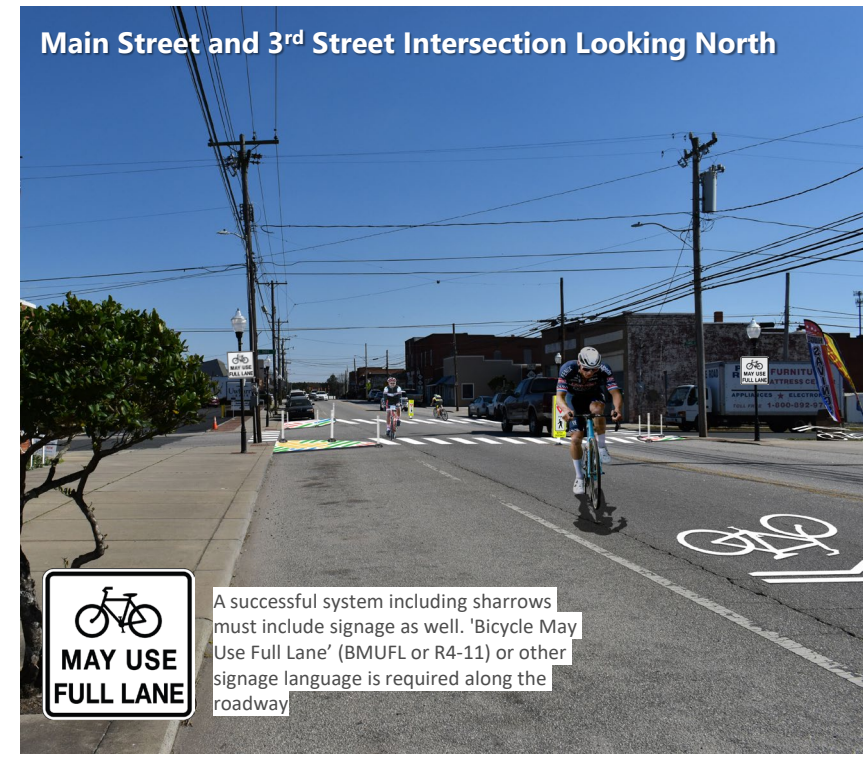
Conceptual rendering of Project BikePed-01 from person-level perspective showing the proposed sharrows and pedestrian crossings with bulb-outs along West Main Street and East Main Street.
