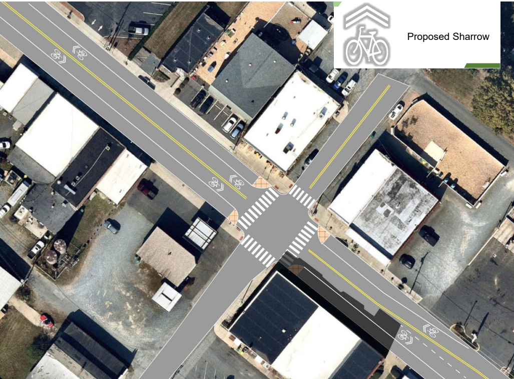
Aerial conceptual rendering of Project BikePed-01, showing the proposed sharrows and pedestrian crossings with bulb-outs along Main Street.
