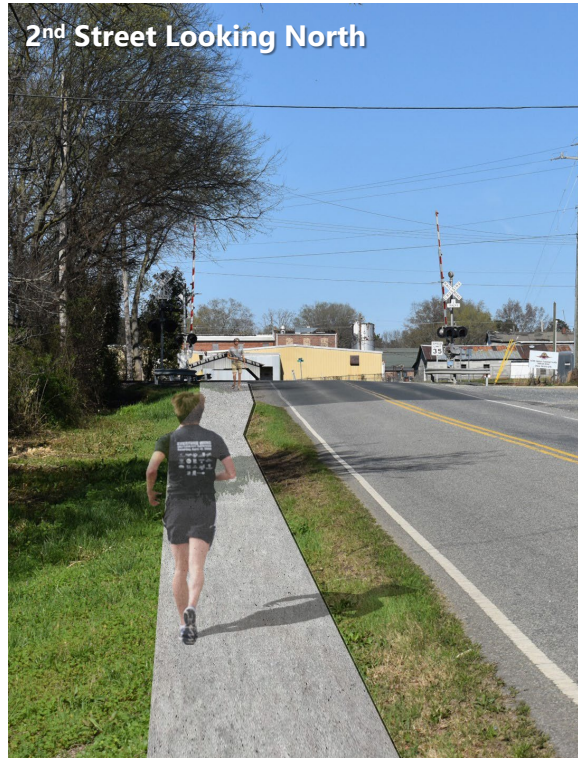
Conceptual rendering of Project SUP-04, Int-06, and Int-16 from person-level perspective showing the proposed shared use path along the west side of 2 nd Street from intersection of Railroad Street to Hamilton Road.
